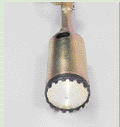
Drilling-crown, extruder in lower position
