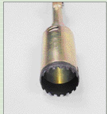
Drilling-crown, extruder in upper position
